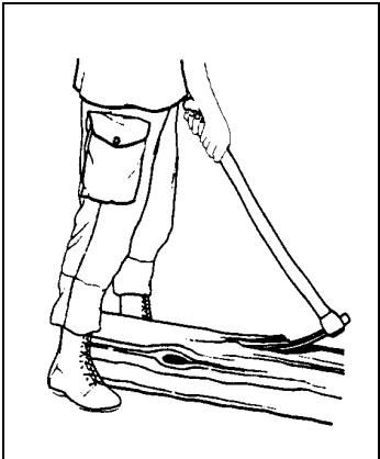
Fig 3-3-7 Correct Method of Using an Adze
