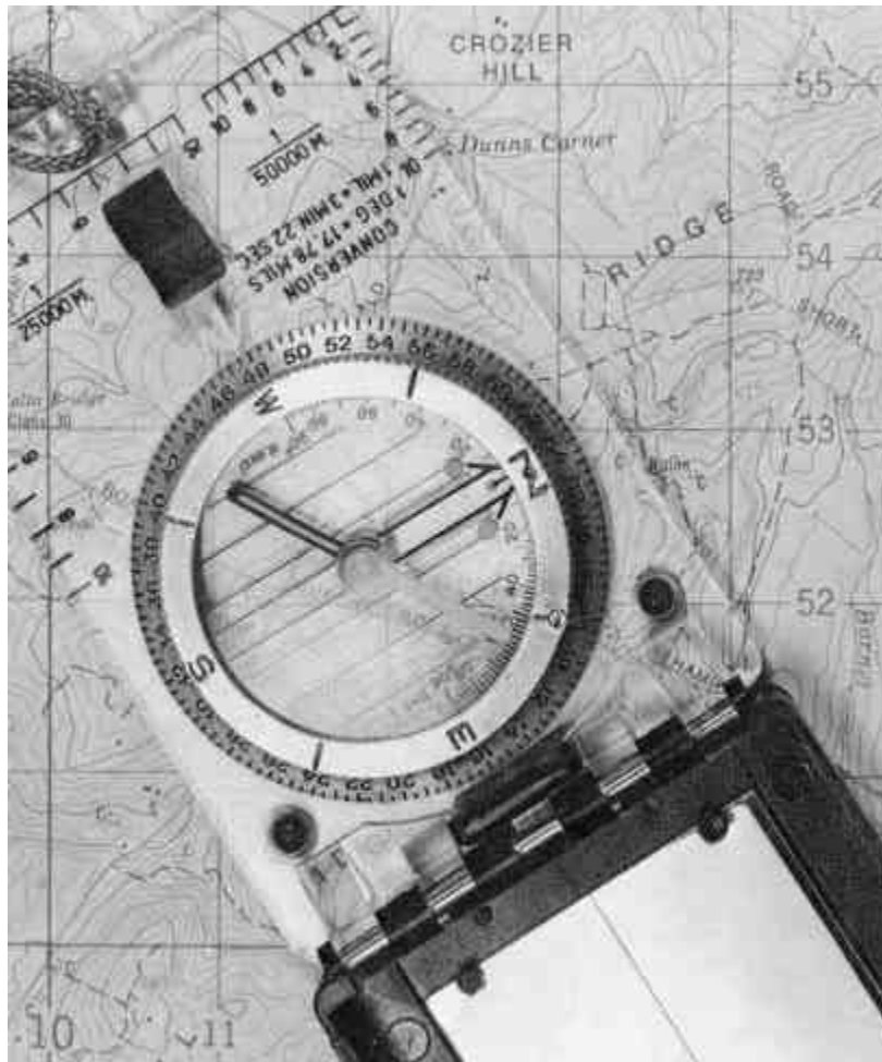
Figure 8-12 The Silva Used as a Protractor
